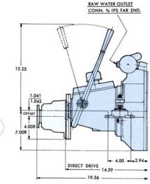
Drawing above shows our WESTERBEKE Short Profile Sailing Gear. This compact 2:1 gear has positive neutral for free-wheeling, and instant acting fingertip control. (Use Morse 33C cable or equal). Weight 25 lb. Turns right hand propeller.
